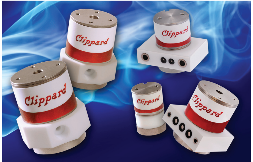
The NIV Series Media Isolation Valves from Clippard are diaphragm or membrane types that are bidirectional and feature all-PTFE wetted areas, as well as the ability to operate in temperatures up to 158°F.
